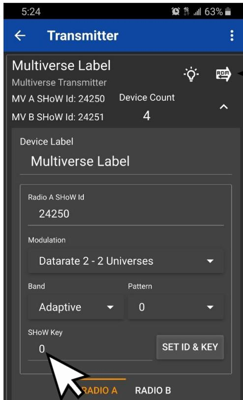
**Figure 7: Setting a SHoW Key with DMXcat**
