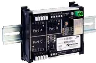
This device allows merging and switching between two DMX sources in a one-universe system. Through the use of automatic signal sensing across four operating modes, any port may detect incoming DMX signals and act as an input and produces two outputs; or two inputs may be merged to create one output; based on priority, HTP merge or switchable using an external contact. The P1017 is RDM discoverable and configured.
