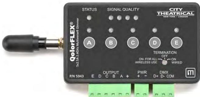
**QolorFLEX® 5x2.5A Multiverse® Dimmers are constant voltage, five-output dimmers that can be controlled wirelessly using City Theatrical’s Multiverse wireless DMX/RDM technology, or legacy SHoW DMX Neo wireless DMX/RDM, or with wired DMX.**
