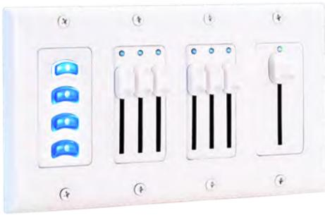
PWWSI Vignette Wall Station, or Vignette™ Sliders and Buttons Wall Stations, is a system of modular button and slider wall station inserts that allow you to snapshot four universes of E1.31 sACN or one universe of DMX512. Design custom wall stations, from single-gang up to six-gang.
