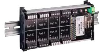
This hub brings flexibility to single universe DMX512 distribution systems. Through use of automatic signal sensing across four operating modes, any port may detect incoming DMX signals and act as an input, or: two inputs may be merged, the user may choose between inputs, or a priority scheme may be invoked. This device is RDM discoverable and configured.
