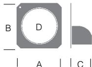
Half Top Hats mask the beam on one side, and allow max light output on the other side. They have a black flocked interior.
