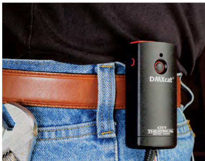
City Theatrical's DMXcat system is designed for use by the lighting professional who is involved with the planning, installation, operation, or maintenance of theatrical and studio lighting equipment. The system consists of a small interface device and a suite of mobile applications. Together, they combine to bring DMX/RDM control plus several other functions to the user's smartphone. DMXcat works with Android, iPhone, and Amazon Fire.
