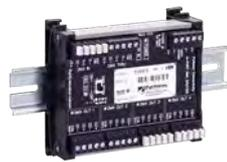
This is an essential part of any permanent DMX512 distribution system. The DIN-rail mountable eDIN Opto-Splitter enables 'star' wiring configurations of DMX512 data lines. Each buffered output is isolated from the DMX input and protects all connected end-devices from harmful electrical faults and ground loops.
