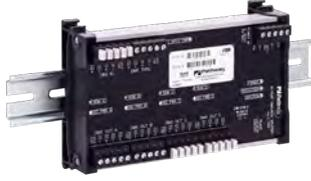
The device provides full isolation between ports and RDM-compatibility. It is a DIN-rail mountable four-way opto-splitter that supports the bi-directional communication standard E1.20 Remote Device Management ("RDM"), as well as DMX512. Used in installations that require 'star' wiring configurations, all output ports are separate electrical entities, fully opto-isolated and independently protected against fault voltages.
