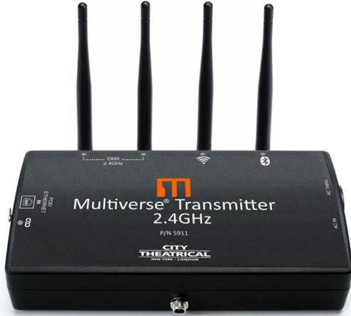
The **Multiverse® Transmitter 2.4GHz (x2)** opens a new world in wireless DMX/RDM. Its Ethernet input allows it to take in Streaming ACN (sACN) or Art-Net and to transmit up to ten user-selectable universes of DMX/RDM, with the ability to use less radio energy than a present-day single universe wireless DMX transmitter.
