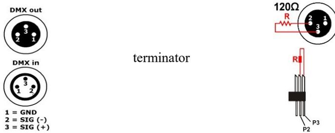
How to turn the controller line from 3-pins into 5-pins (plug and socket).
