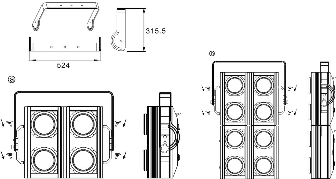
Fixture jointing (Between more than two units)
