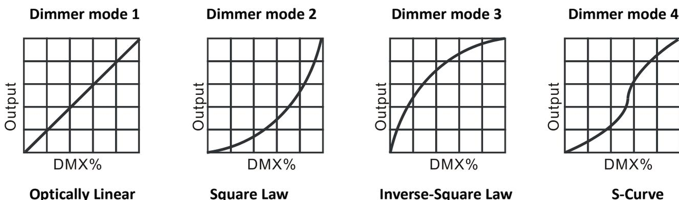
Mode 1(Optically Linear): The increase in light intensity appears to be linear as DMX value is increased.
