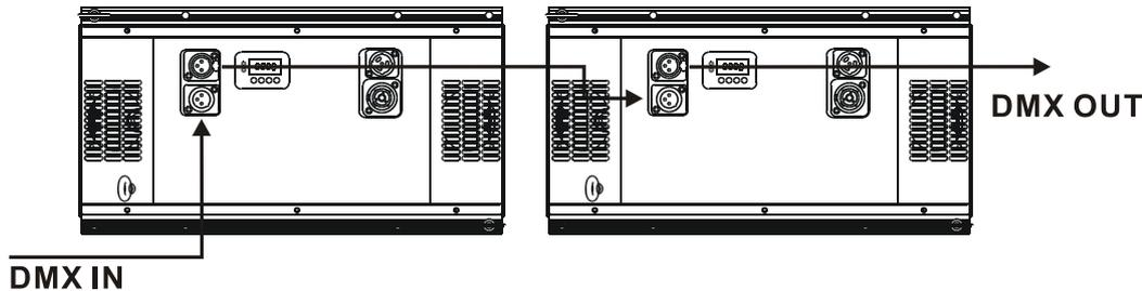
1. Connect the fixture together in a “daisy chain” by XLR plug cable from the output of the fixture to the input of the next fixture. The cable cannot be branched or split to a “Y” cable. Inadequate or damaged cables, soldered joints or corroded connectors can easily distort the signal and shut down the system
